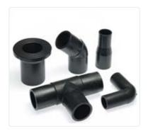
Uponor's electrofusion fittings product range includes sockets, reducers, bends, T-branches, drilling saddles and plugs. These fittings are welded using a electrofusion machine, which passes an electrical current to the fitting via resistance wires, thus heating the fitting and fusing it to the pipe. This method is being increasingly adopted, especially for the jointing of small diameter pipes.
